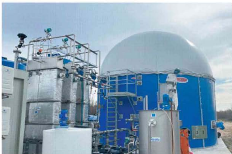
FIGURA 2. BIORREACTOR ANAERÓBICO Y SET DE MEMBRANAS FIGURE 2. ANAEROBIC BIOREACTOR AND MEMBRANE SET
